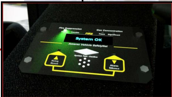
SafetyNet Display Panel
