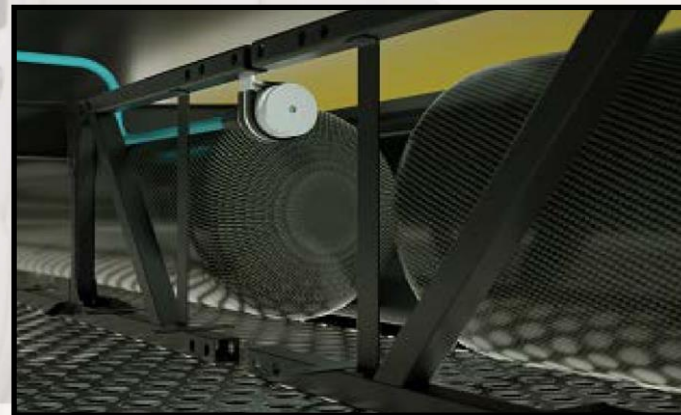
Gas Sensor in cylinder compartment
